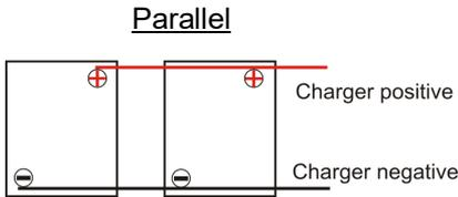
When batteries are connected in Parallel the battery amp hour capacity is additive and the voltage remains the same.
