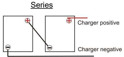
When batteries are connected in Series the voltage is additive and the battery amp hour capacity remains the same.
