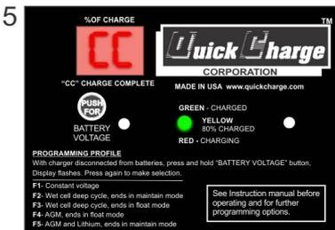
Shortly after the cycle reaches 99%, the cycle terminates and displays CC "Charge Complete". The LED will be solid green if the charger is set to maintain mode, or flicker if set to float mode.
