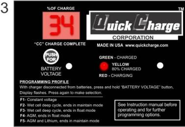
As the cycle progresses, the display indicates the progress. Here the cycle is 34% complete.
