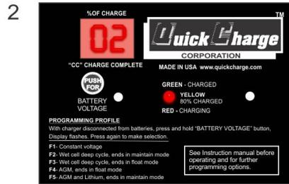
After displaying the profile for a few seconds, the LED will turn solid red, and display 02 on a discharged battery. The time it spends there depends on how deeply discharged it is, it may be hours before it starts to move higher, or seconds if the batter is already charged.
